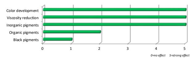
**UNIQ** \*\*SPERSE P-144 is a wetting and dispersing additive for filled unsaturated polyester, acrylic and epoxy resins to reduce the viscosity and prevent settling. Strong viscosities reduction so higher pigment and filler loading in the grinding process can be achieved. For fiber-reinforced spray up and hand lay-up resins.
